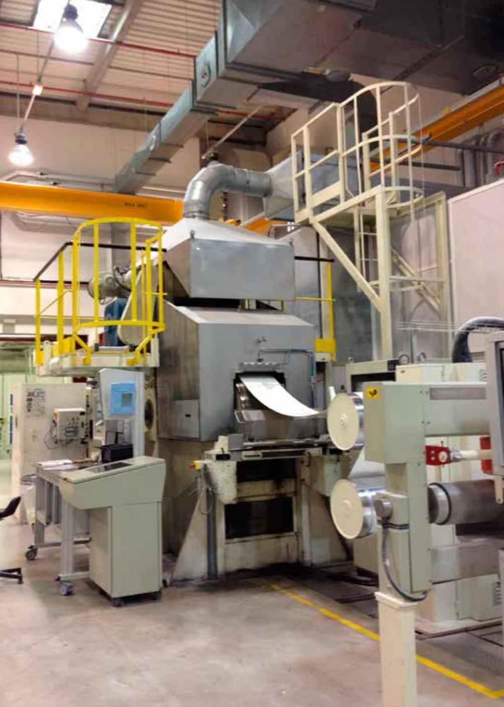
One of Aptar's Rotocures vulcanizes a rubber band to change its molecular structure for making rubber washers.
