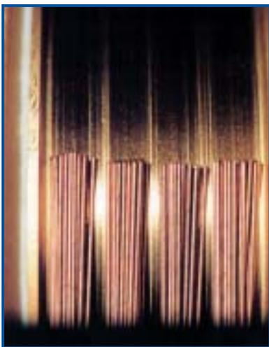
simply a group of individual metal fibers (wires) that are collimated by and terminated into a metal tube as illustrated in the photo on the left. In this cantilevered design, the free, unterminated end of the fiber brush bundle rides in a groove on the ring surface.
