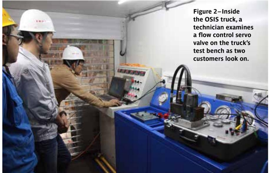
**Figure 2—Inside the OSIS truck, a technician examines a flow control servo valve on the truck's test bench as two customers look on.**
