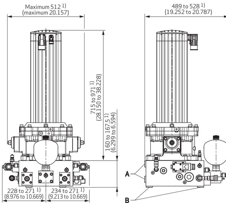
A: Distance washer for radial connection<sup>1)</sup>
