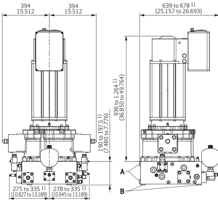
A: Distance washer for radial connection <sup>1)</sup>
