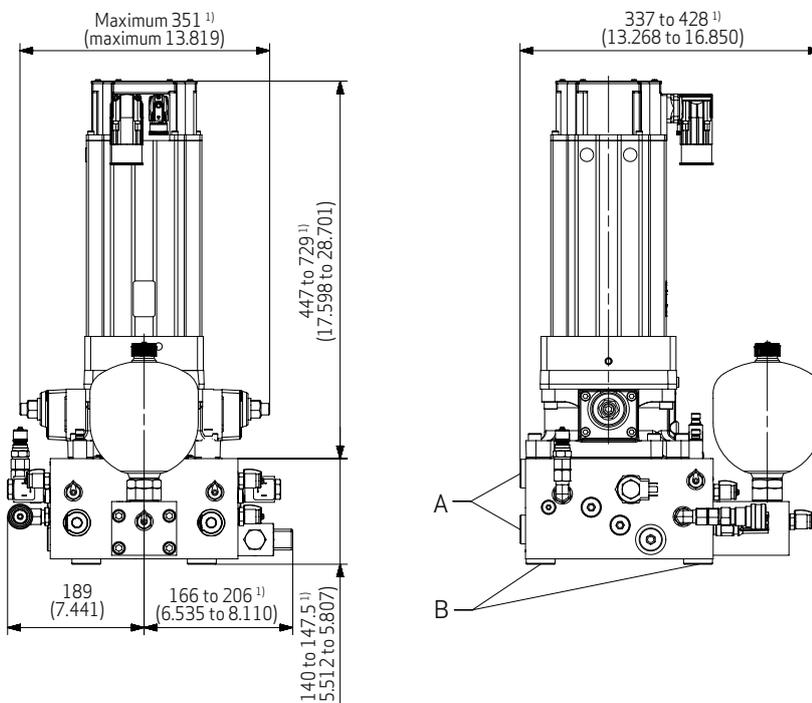
A: Distance washer for radial connection <sup>1)</sup>
