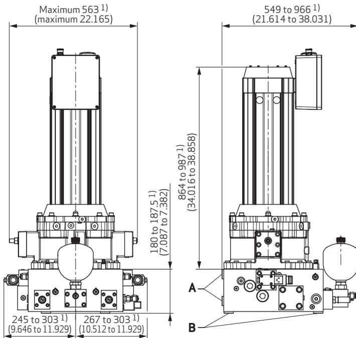
A: Distance washer for radial connection <sup>1)</sup>
