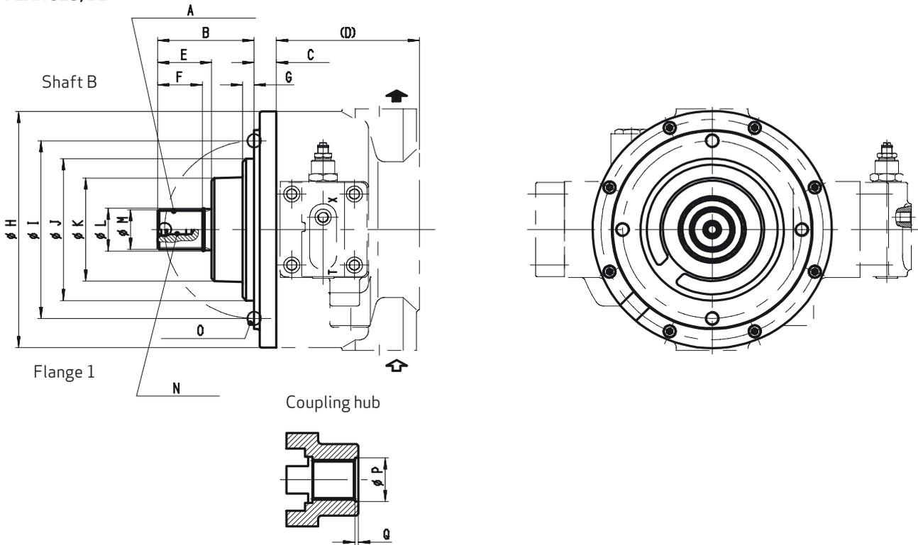
Involute spline according to DIN 5482 (for B1)
