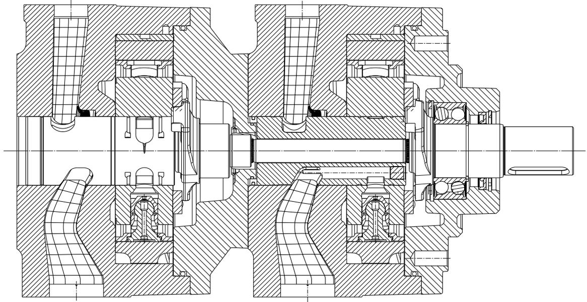
Radial piston pump with tandem-mounted gear pump using SAE-A adapter
