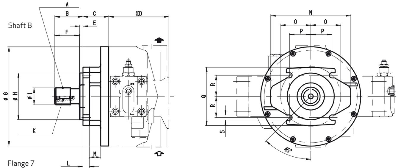
Involute spline according to DIN 5480
