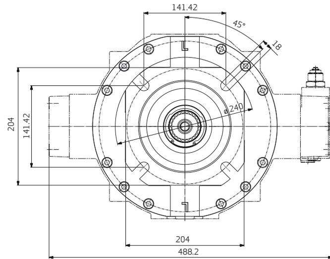
Involute spline according to DIN 5480 (for RKP mounting obligatory)
