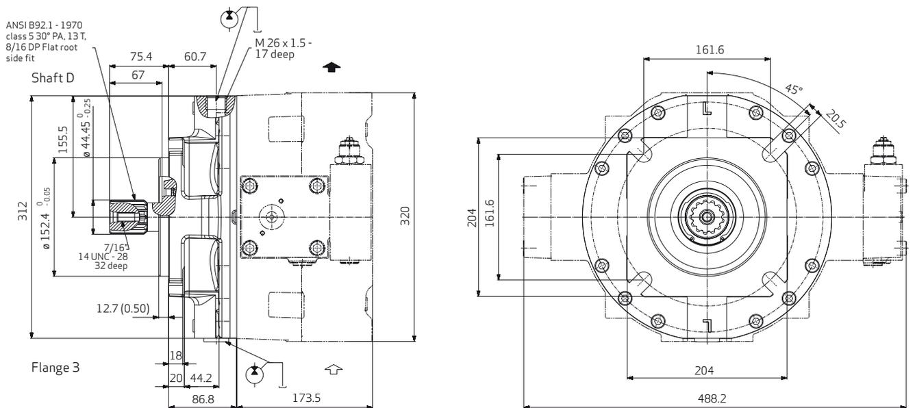
Involute spline according to SAE 744 C (for RKP mounting obligatory)
