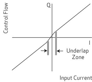
Normally used in hydraulic motor applications
