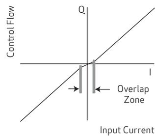
Normally used in failsafe applications
