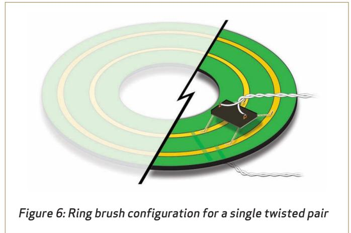
**Figure 6: Ring brush configuration for a single twisted pair**
