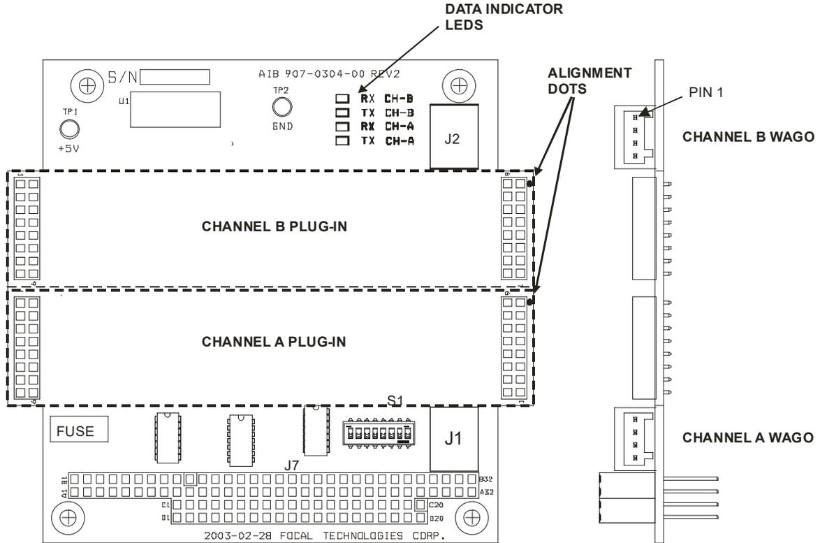
Figure 2-5: 907-AIB Adapter Card
