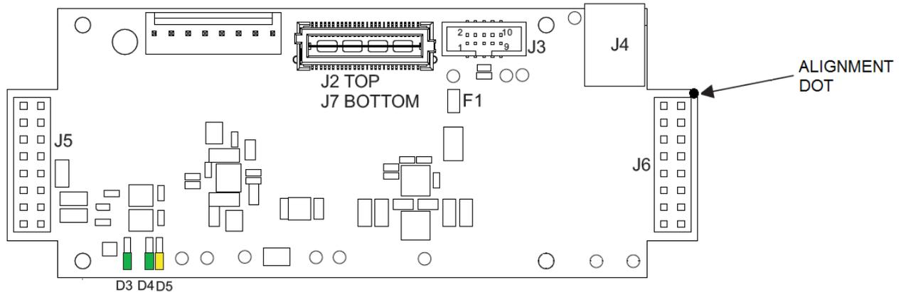
**Figure 2-7: 914-AX AIB Adapter Card**
