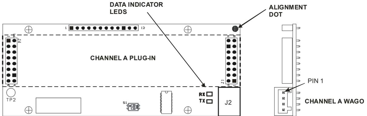
**Figure 2-6: 914-AIB Adapter Card**
