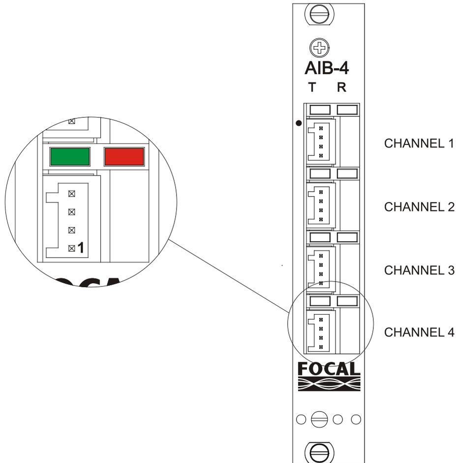
Figure 2-1: Model 903 AIB-4 Front Panel
