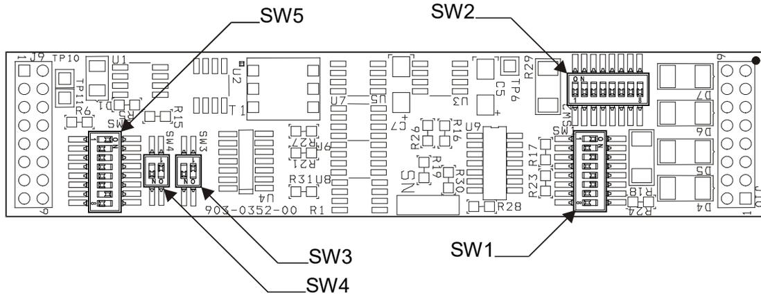
Figure 4-2: AIB RS-485 Plug-In Module
