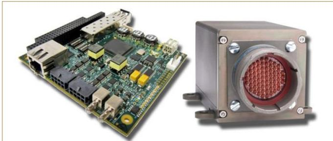
*Figure 20: Two examples of multiplexers are shown. A board level multiplexer that supports multiple uncompressed HD video channels, multiple serial data channels and a single Gigabit Ethernet port. A small Camera Link® multiplexer is shown that converts copper Camera Link signals into a single fiber channel.*
