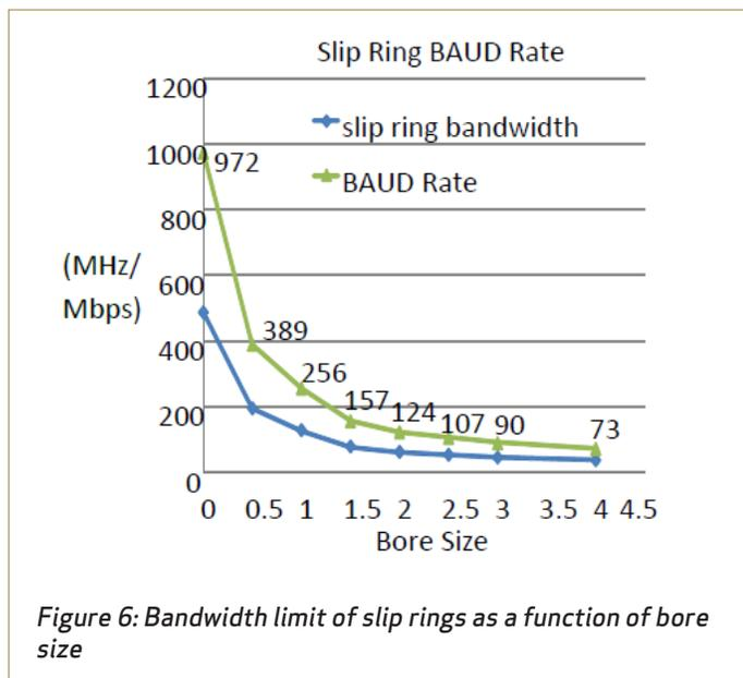
This length (or diameter) effect can be minimized by minimizing the impedance mismatch between the discontinuity and the transmission line, but it is impossible to completely eliminate. The two insertion loss plots of Figure 7 are of data channels that are identical except for diameter. The top rings are approximately 6.4 cm in diameter and the rings in the bottom chart are approximately 15 cm in diameter. The critical diameter calculations graphed above would tell us that these rings
