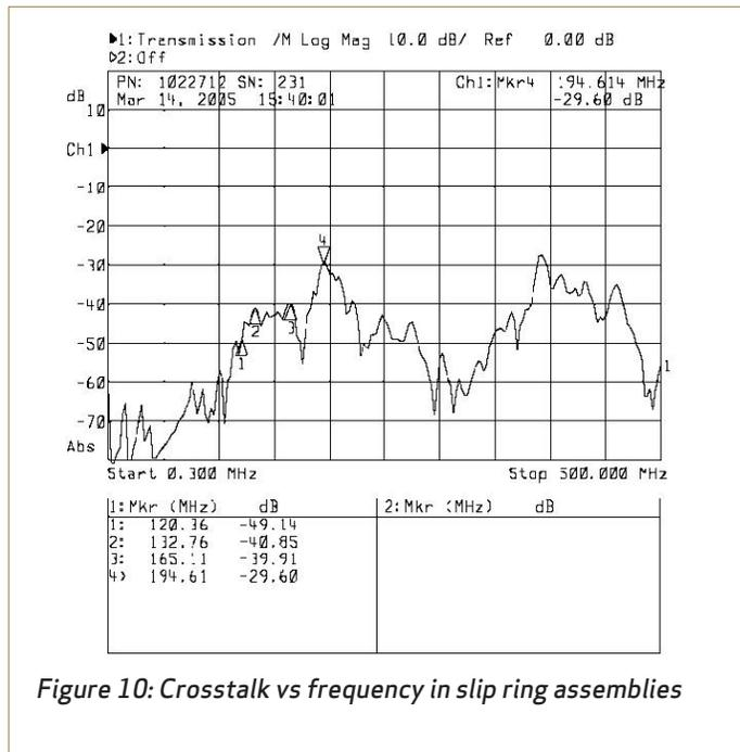
Figure 10: Crosstalk vs frequency in slip ring assemblies
