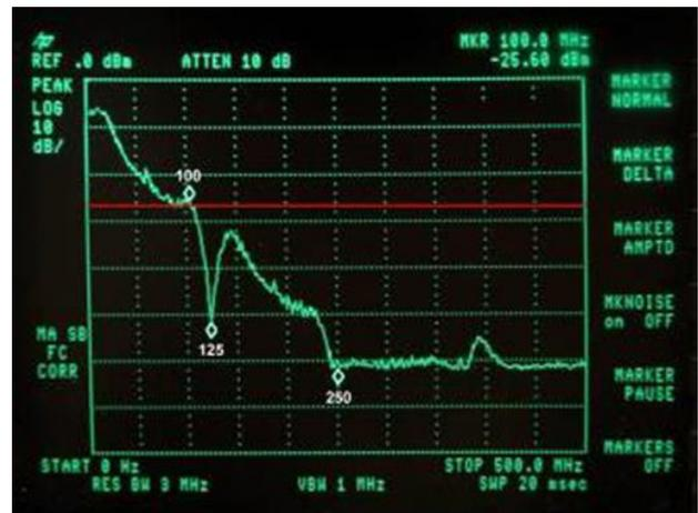
Figure 4: Frequency spectrum of 100Base-T Ethernet
