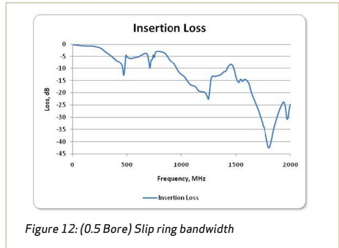
The data show that the resonances in transmission line are complex and there is little value in trying to look past the -6 dB point. This data, along with other tests and evaluation, leads us to the conclusion that the estimates represented by Figure 6 are somewhat conservative and a useful method of predicting usable bandwidth of a slip ring of known diameter.
