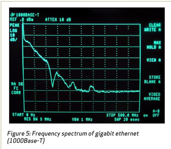
Figure 5: Frequency spectrum of gigabit ethernet (1000Base-T)
