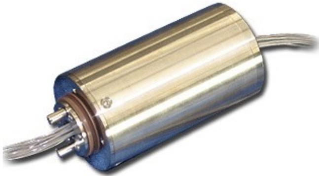
The FO300 is a prism based multichannel fiber-optic rotary joint (FORJ). It is a passive and bidirectional device which can be used as a standalone device or easily integrated into a rotary assembly, enabling transfer of high data rate optical signals across a rotating interface.
