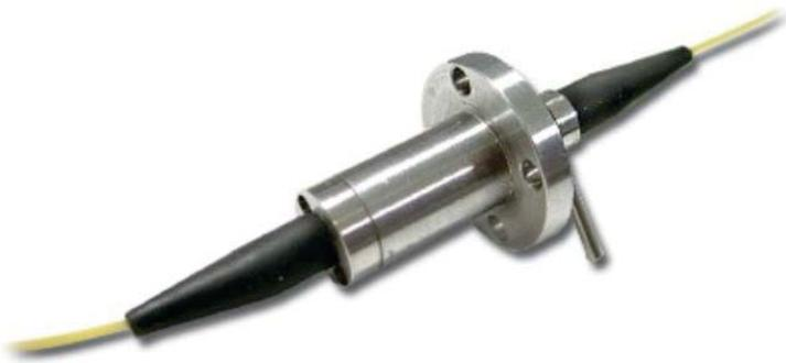
The FO285 (single-channel singlemode) and the FO286 (single-channel multimode) are passive and bidirectional, and allow the transfer of optical signals across rotational interfaces. Both models also offer other benefits of fiber optics, including low spark hazard.
