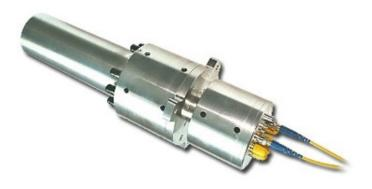
The FO291 is a multi-pass, singlemode fiber optic rotary joint (FORJ). It is passive and bidirectional, and allows the transfer of optical signals across a rotational interface on 2 to 9 separate singlemode optical fibers.
