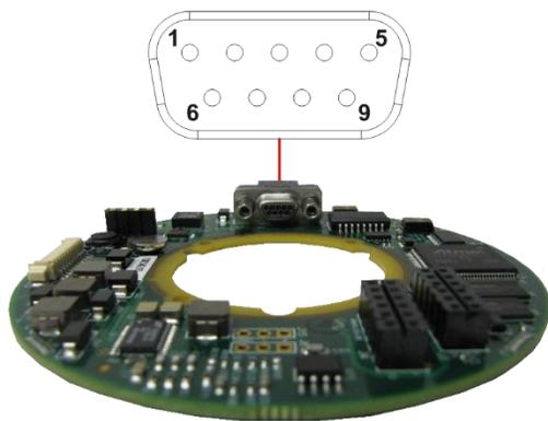
**Figure 5-1: Micro-D (9-pin) Power & Data Connector (J5)**
