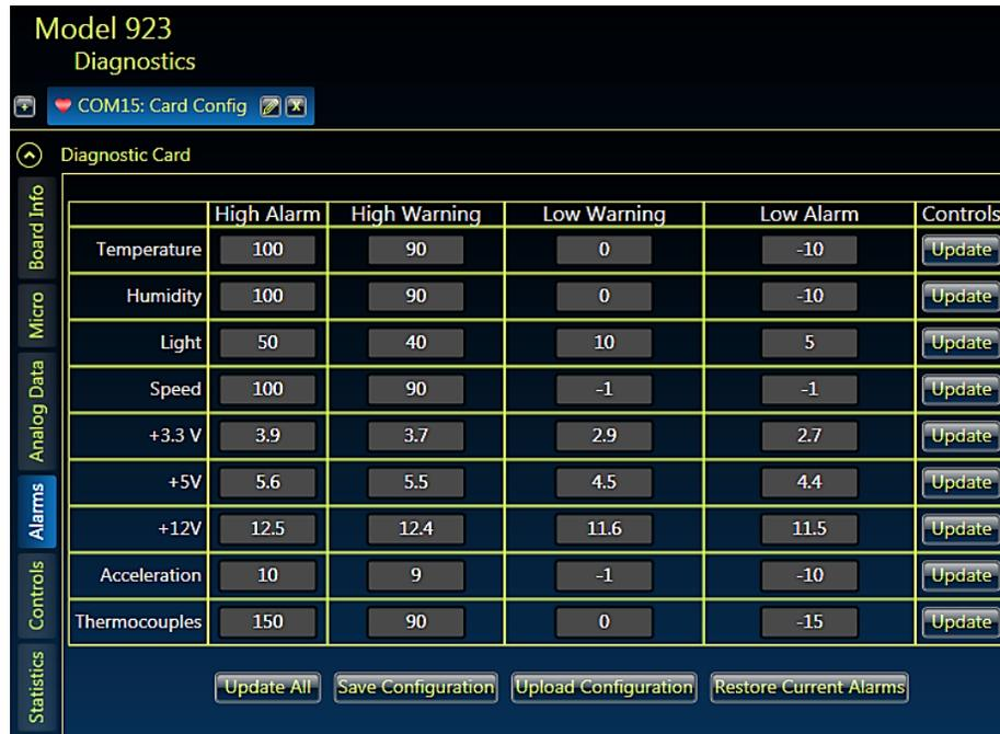
**Figure 6-6: 923-GUI – Alarm Configuration**
