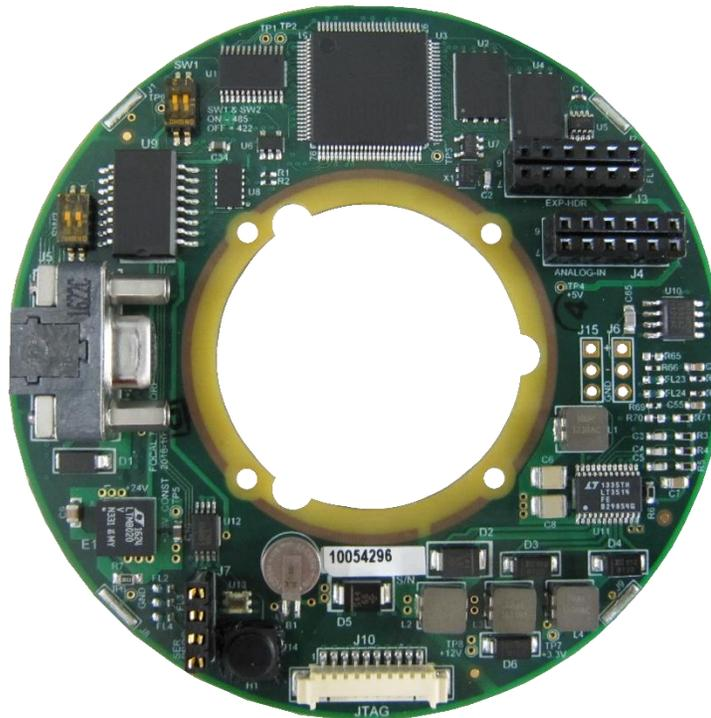
Figure 1-1: Model 923 Electronic Data Logger Card
