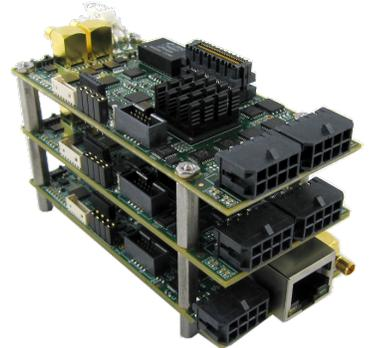
All 914-X Series cards include advanced serial diagnostics and configuration interfaces. This facilitates easy configuration of the cards without requiring physical access, as well as easy to display system status. The same interface can be used to update the system firmware or to upgrade the feature set with higher speed interfaces and new expansion possibilities. LED headers simplify integration with cost effective enclosure diagnostic LEDs.
