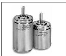
As a circuit element, the synchro is essentially a variable-coupling transformer; the magnitude of the magnetic coupling between the primary and secondary, and hence the magnitude of the output voltage, varies according to the position of the rotatable element. In function, the synchro is an electromechanical transducer. A mechanical input such as a shaft rotation is converted to a unique set of output voltages, or a set of input voltages is used to turn a synchro rotor to a desired position.
