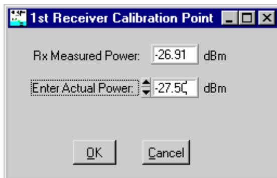
**Figure 11** - Receiver Calibration Window (1st Point)
