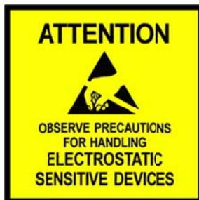
Grounded ESD wrist straps must be worn and proper ESD safety precautions observed when handling printed circuit boards.
