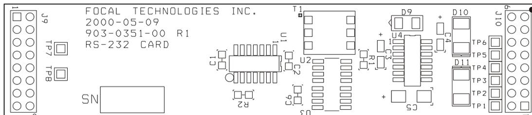
**Figure 4-11: AIB RS-232/TRIGGER Plug-In Module**
