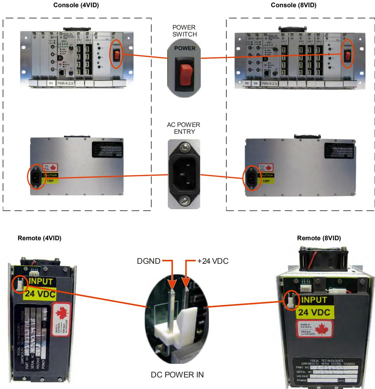
Figure 3-10: Power Connectors Location (4VID and 8VID Systems)
