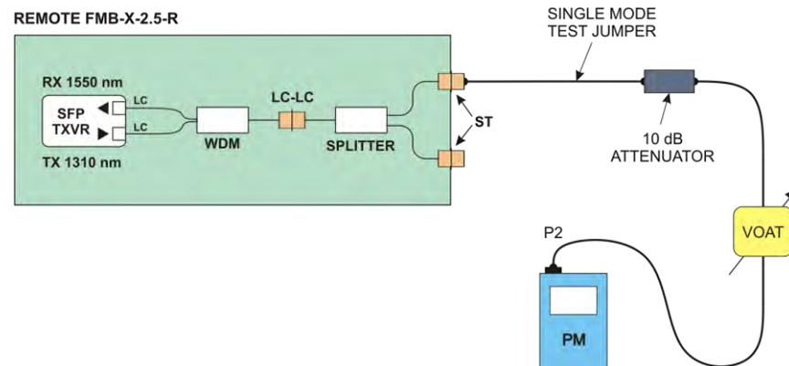
**Figure 6-7: Power Budget Test Setup – Received Sensitivity Measurement**
