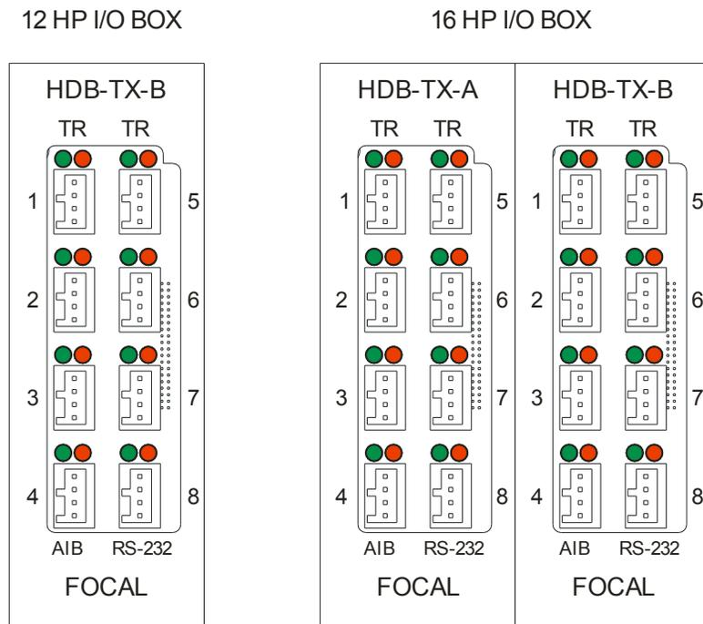
Figure 4-4: I/O Interface Box for 12 HP and 16 HP High Density Remote Systems
