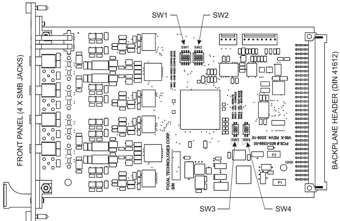
**Figure 4-7: VIB-X Plan View**
