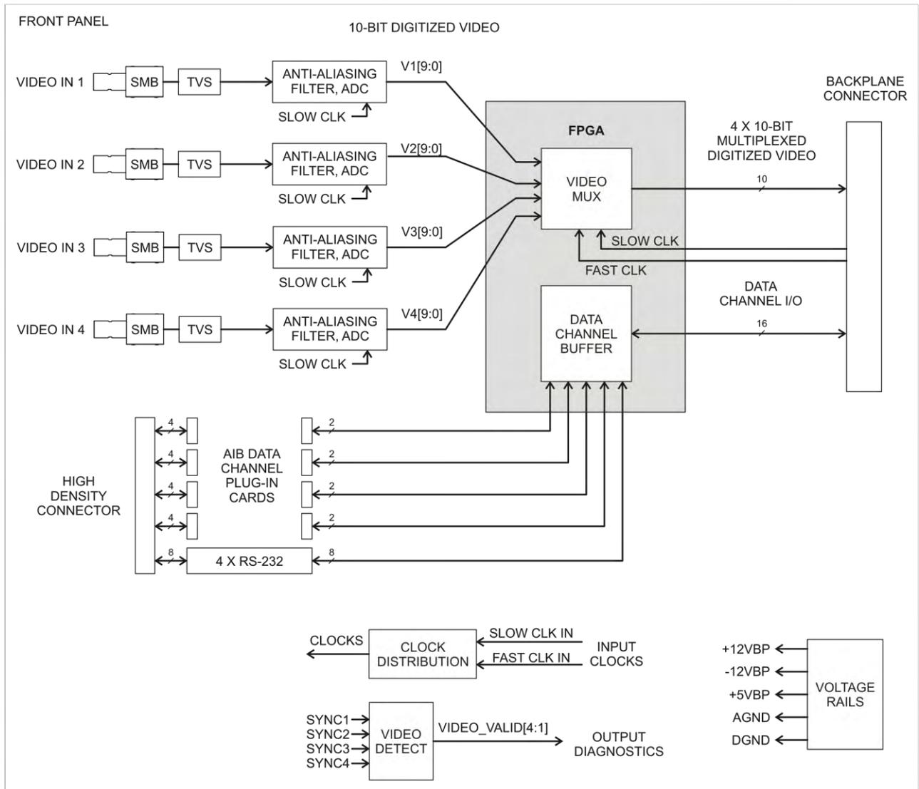
Figure 4-3: HDB-TX Block Diagram
