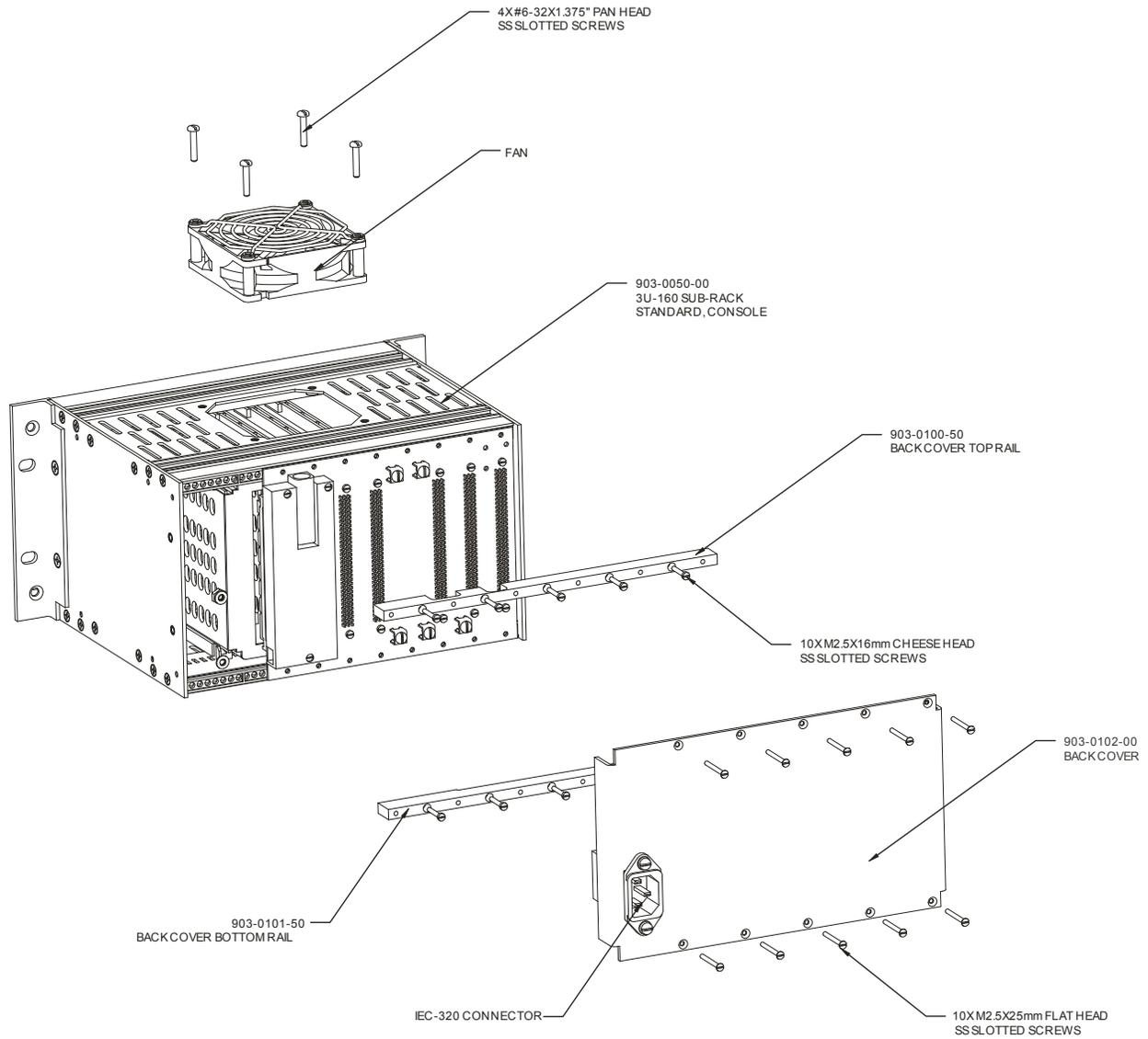
Figure 6-2: Exploded View of a Model 903 4VID Console Card Cage
