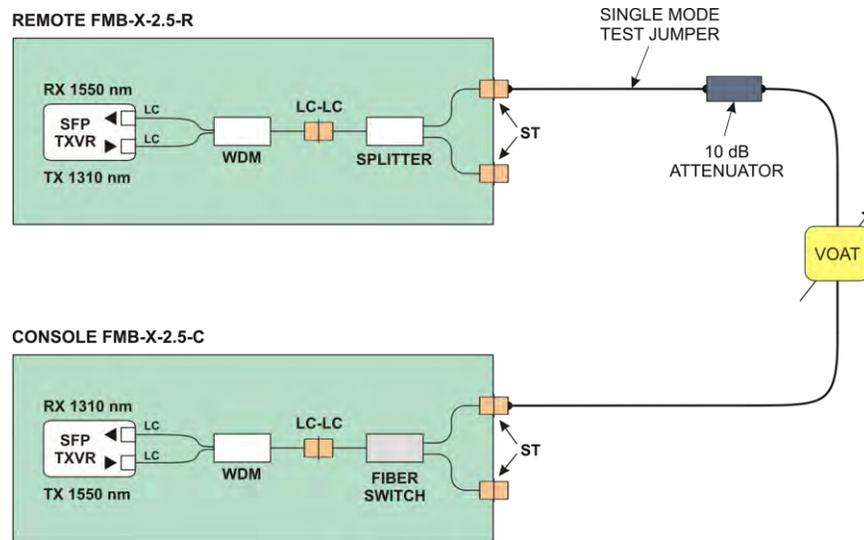
**Figure 6-6: Power Budget Test Setup – Link Threshold Measurement**
