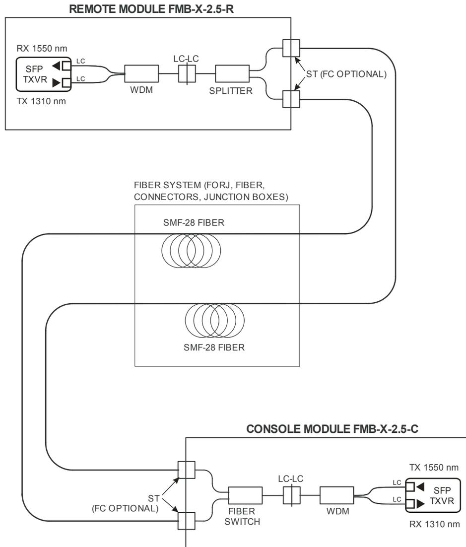
**Figure 2-7: Model 903 Dual Fiber Optic Transmission System (4VID, 8VID)**
