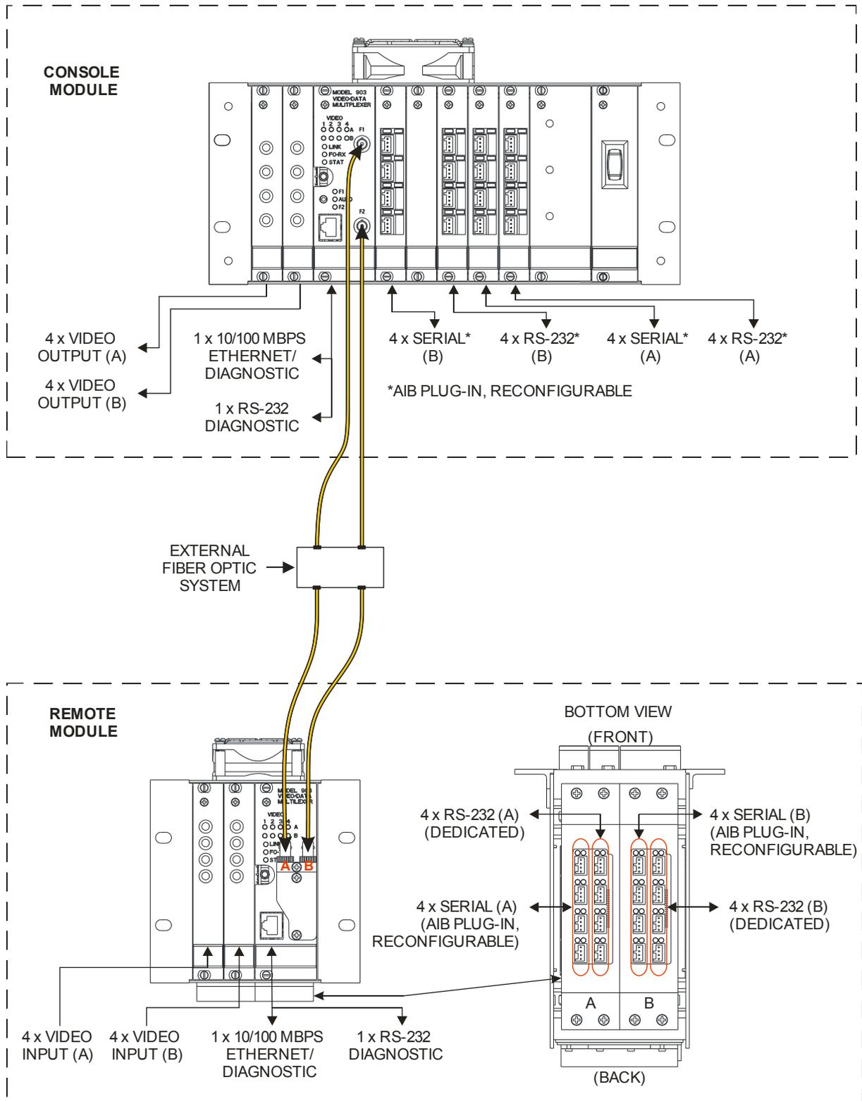
Figure 2-2: Model 903-HD Multiplexer – I/O Ports (8VID System)
