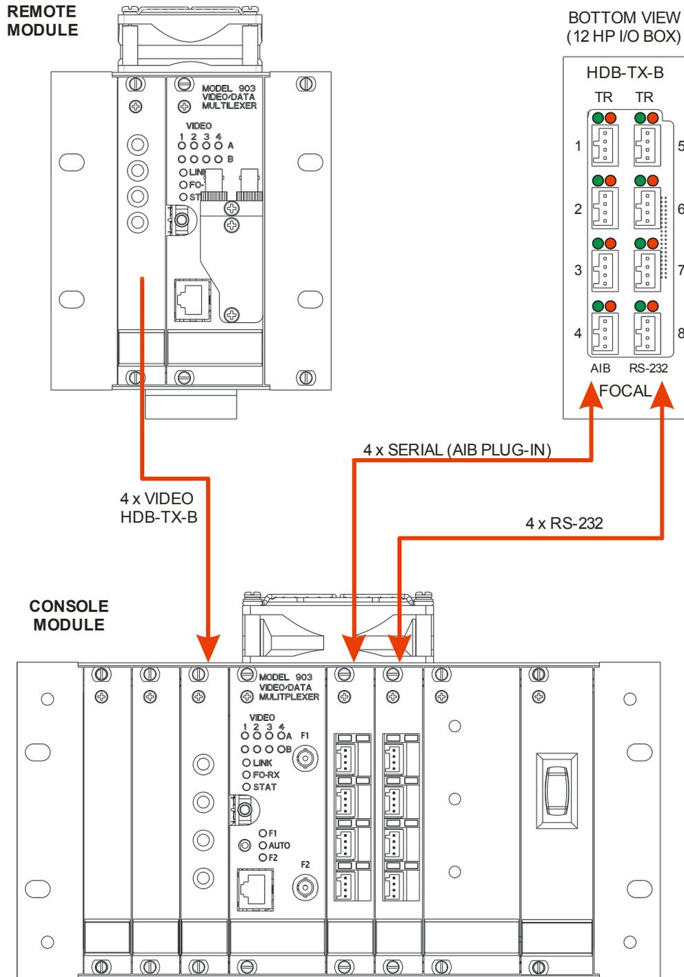
Figure 2-5: Console and Remote Modules (4VID) Showing Slot Pairings for Video and Data
