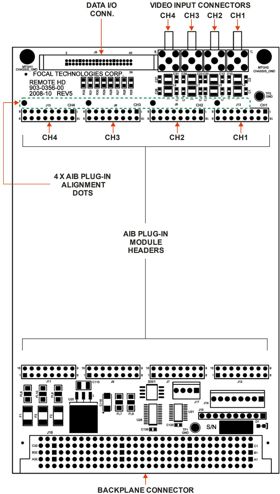
Figure 4-2: HDB-TX PCB and Connector Location
