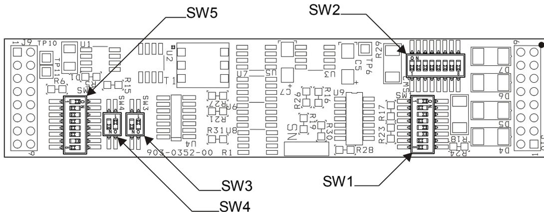
**Figure 4-12: AIB RS-485 Plug-In Module**
