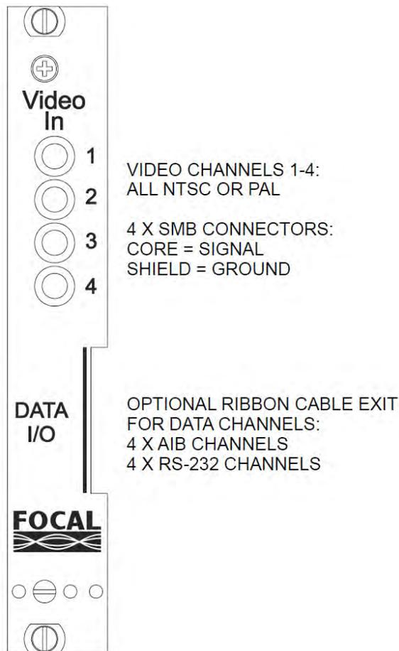
Figure 4-1: Remote High Density Board (HDB-TX) – Front Panel
