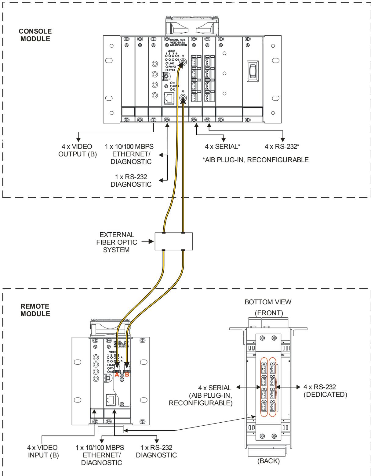
Figure 2-1: Model 903-HD Multiplexer – I/O Ports (4VID System)
