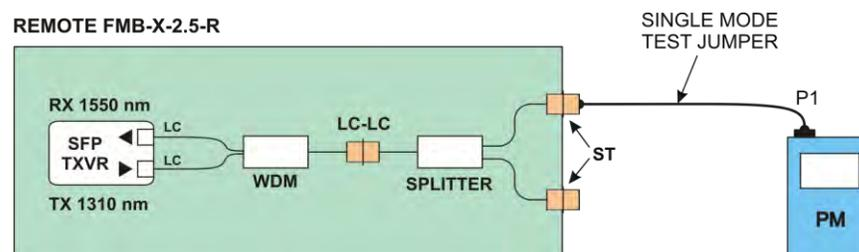
**Figure 6-5: Power Budget Test Setup – Transmit Optical Power Measurement**
