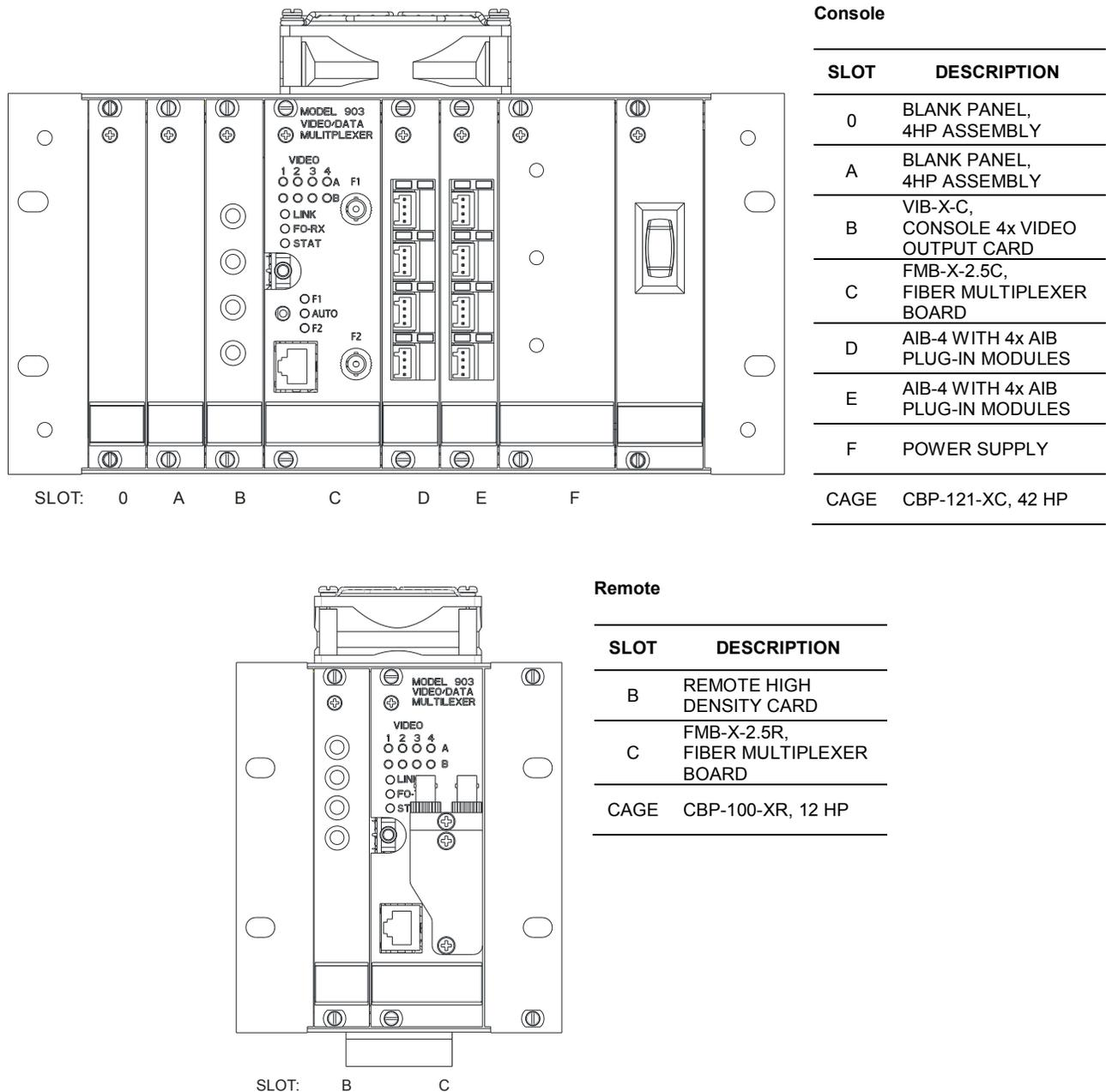
Figure 2-3: Model 903-HD Mux Front Panel View – Card Configuration (4VID)
