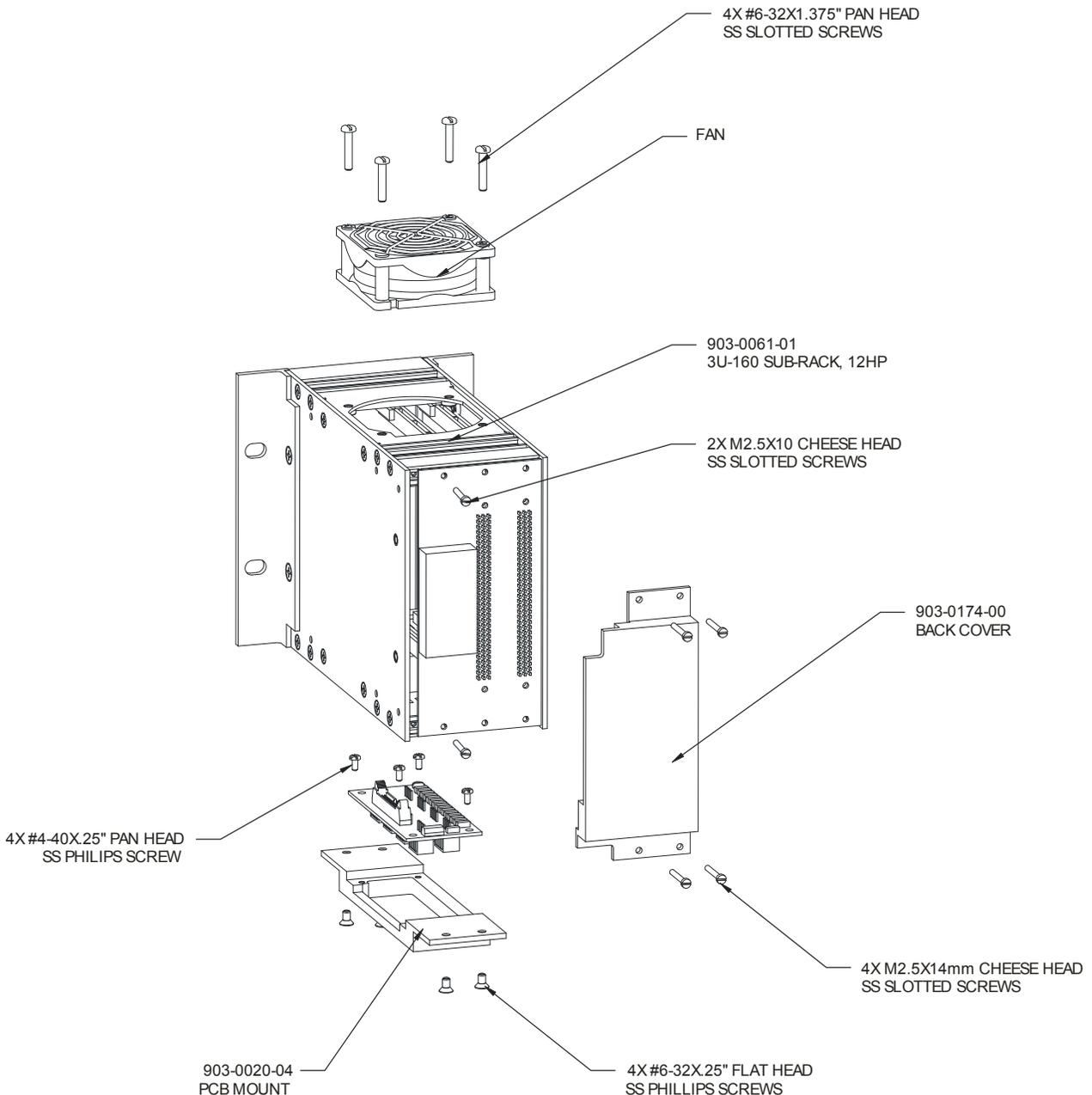
**Figure 6-4: Exploded View of a Model 903 High Density 4VID Remote Card Cage**
