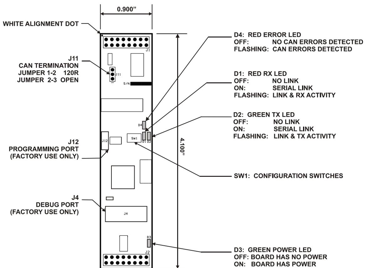
Figure 4-17: AIB-CANBUS Plug-In Module (Top View)
