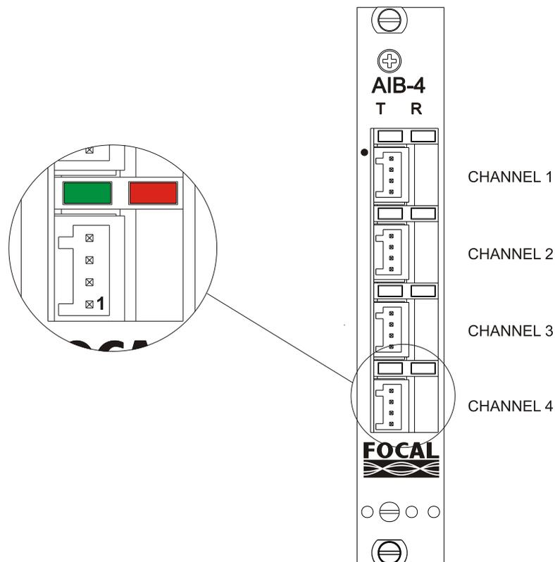
Figure 4-8: Adaptable Interface Board (AIB-4) Front Panel
