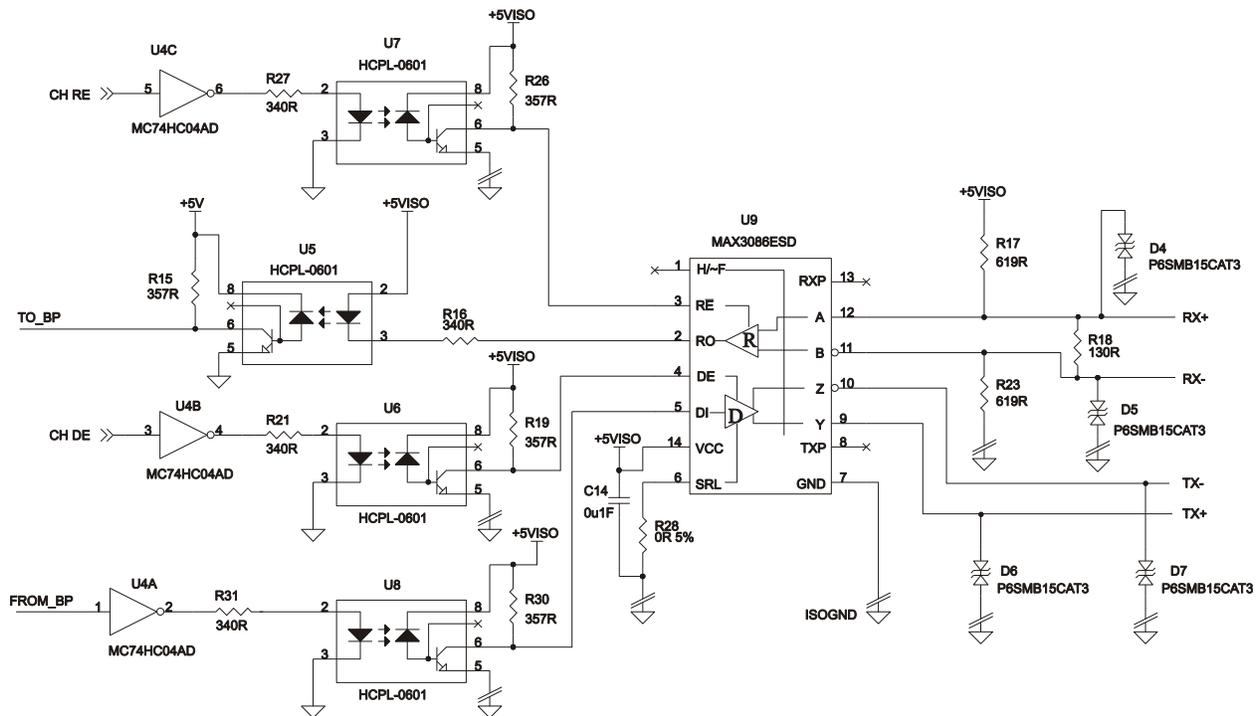
Figure 4-13: AIB RS-422 Interface Schematic
