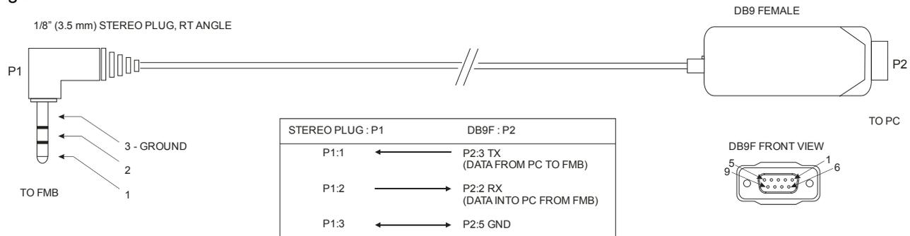
**Figure 3-4: FMB-X-2.5 RS-232 Diagnostic Cable: 1/8" (3.5 mm) Stereo to DB9F**
