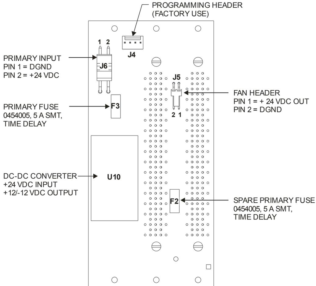
Figure 3-8: 12 HP High Density Remote Backplane PCBA (+24 VDC Input)
