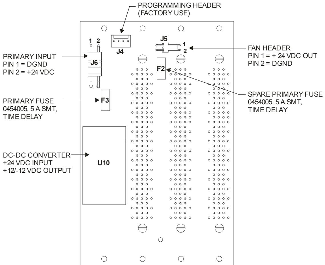
Figure 3-9: 16 HP High Density Remote Backplane PCBA (+24 VDC Input)
