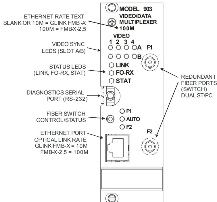
Figure 3-3: Console FMB-X-2.5 Front Panel
