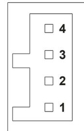
Pin assignments for the WAGO connectors used with the I/O-Box and AIB-4 cards are given in the table below for RS-232 and RS-485. The dedicated RS-232 channels on the I/O-Box include opto-isolated data lines and separate isolated power/ground per channel. Also, each AIB-232 or AIB-485 plug-in module includes opto-isolated data lines and separate isolated power/ground per channel. **Refer to appendix A for more information about the connector part numbers and pin assignments.**
