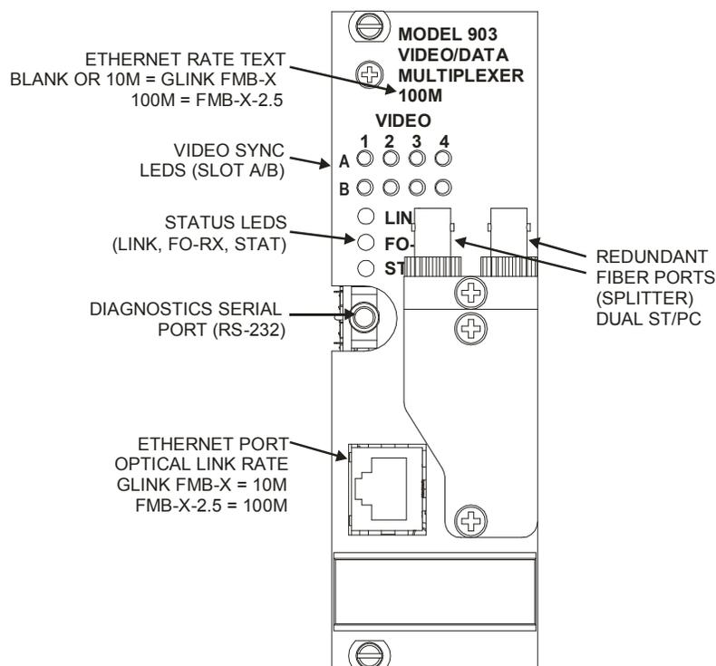
Figure 3-1: Remote FMB-X-2.5 Front Panel View
