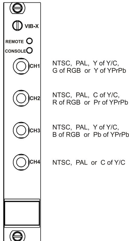
Figure 4-5: VIB-X Front Panel
