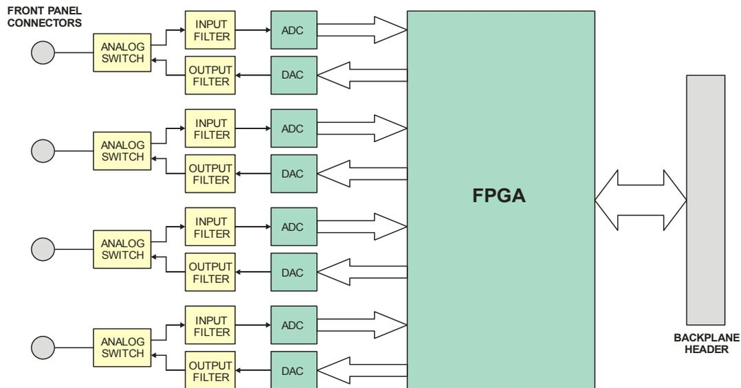
Figure 4-6: Block Diagram of VIB-X Card
