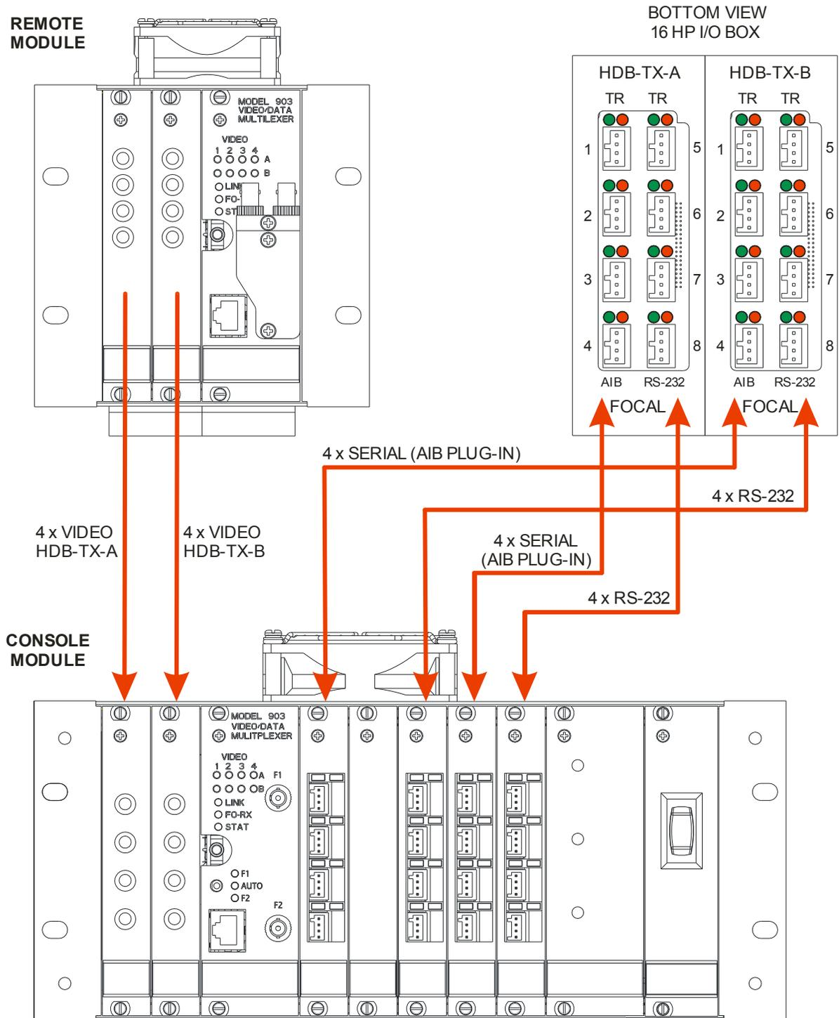
Figure 2-6: Console and Remote Modules (8VID) Showing Slot Pairings for Video and Data
