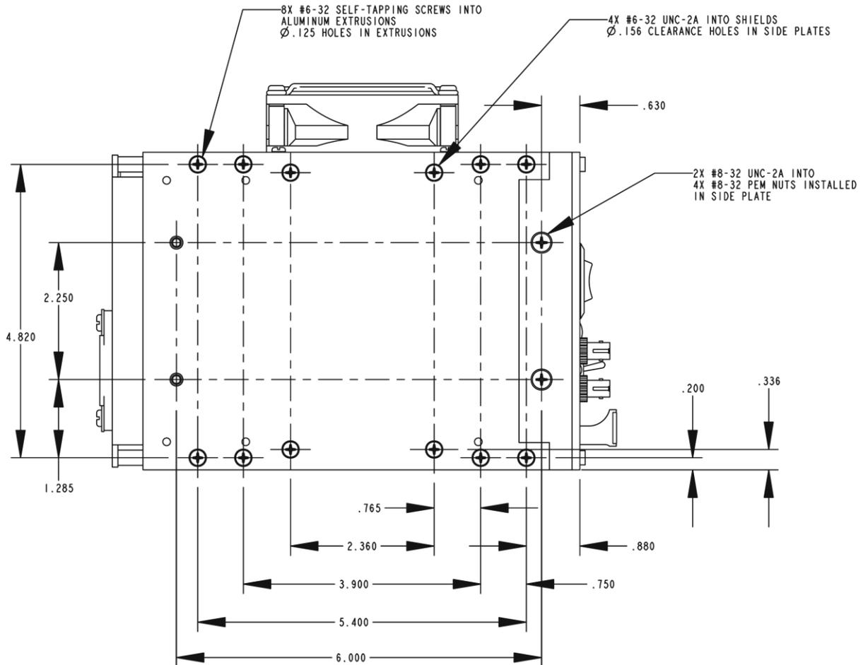
**Figure 6-1: Side View of Typical Model 903 Console Card Cage.**
