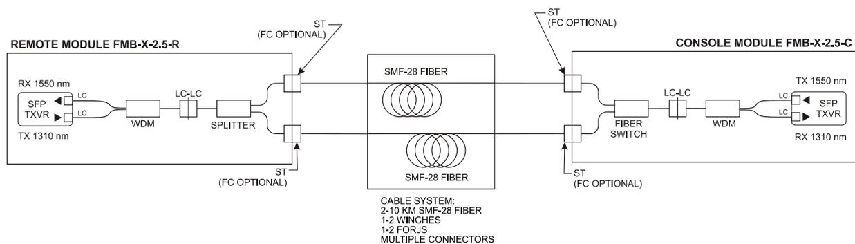
**Figure 5-1: Block Diagram of Model 903 Fiber Optic Transmission System**
