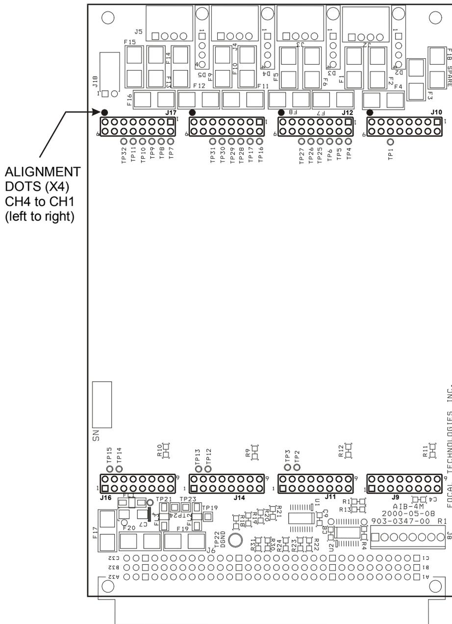
Figure 4-9: Adaptable Interface Board (AIB-4) PCB
