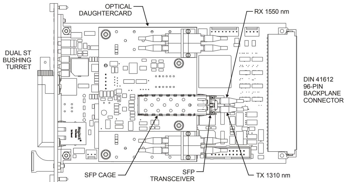
**Figure 3-2: Remote FMB-X-2.5 Plan View**
