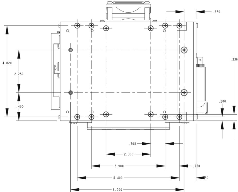
**Figure 6-3: Side View of Typical 16 HP Model 903-HD Remote Card Cage.
