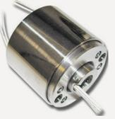
303 Miniature Bore             | Up to 600 rpm standard<br>Contact factory for other requirements | Up to 230° C (200 °C standard) | 25 kpsi (1,700 bar) | Up to 8  | 250 - 500 VAC standard | Up to 2 A per channel | 0.375 in. (9.525 mm) hollow bore ID, -1.7 in. (43.2 mm) minimum OD |
