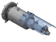
M140 EX3-1 + ESR 110 / 32-1+LWL-QC [20079]   | 32       | Max. 230 volt | Max. 20 amps  | 3 x Ethernet; 1 x optical channel | Connectors   | 2x hydraulic oil at max. 280 bar; 1x gear oil at max. 16 bar | For 6.0 MW turbine                                          |
