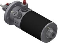
Rotoflux ESR 70 [24400] + air channel G 1/4" (at max. 10 bar)   | Max. 24  | Max. 480 volt | Max. 20 amps | PROFIBUS®,<br>CAN Bus,<br>Ethernet,<br>DeviceNet™,<br>PROFINET® | Cable (standard),<br>max. 10 m | 6.91 - 8.17 x Ø2.76<br>(175.5 - 207.5 x Ø70) | IP 64,<br>max. 200 rpm |
