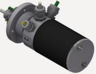
Rotoflux ESR 70 [24400]                                         | Max. 24  | Max. 480 volt | Max. 20 amps | PROFIBUS®,<br>CAN Bus,<br>Ethernet,<br>DeviceNet™,<br>PROFINET® | Cable (standard),<br>max. 10 m | 6.28 - 7.54 x Ø2.76<br>(159.5 - 191.5 x Ø70) | IP 64,<br>max. 200 rpm |
