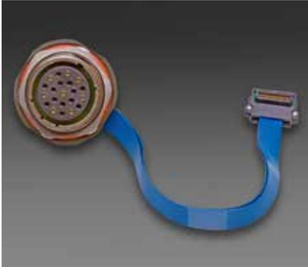
Moog Protokraft Lightning series fiber optic transceivers integrate multiple fiber optic transmitter and receiver functions into a MIL-DTL-38999 series III receptacle connector.
