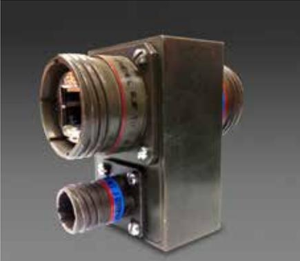
Moog Protokraft Saturn series fiber optic Ethernet media converters consist of optoelectronic transmitter and receiver functions integrated along with the 10/100Base-TX to 100Base-FX or 1000Base-T Ethernet electrical to 1000Base-LX or 1000Base-SX Ethernet optical media conversion circuitry into an environmentally sealed unit.
