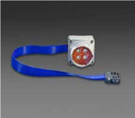
Moog Protokraft Dagger series D38999 transceivers, transmitters and receivers consist of optoelectronic transmitter and receiver functions integrated into a wall mount D38999 cylindrical connector. The optical transmitters are 850 nm VCSEL lasers. The transmitter input lines are driven with differential CML signals applied to the transmitter (TX+ and TX-) lines. Dual loop, temperature compensated, VCSEL drivers convert the transmitter input signals to suitable VCSEL bias and modulation currents.
