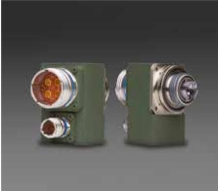
Moog Protokraft Maverick series fiber optic Ethernet media converters consist of optoelectronic transmitter and receiver functions integrated along with the 10/100Base-TX to 100Base-FX or 1000Base-T Ethernet electrical to 1000Base-LX or 1000Base-SX Ethernet optical media conversion circuitry into an environmentally sealed unit.
