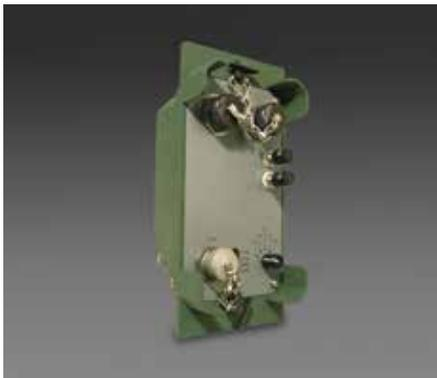
The 108600 converts digital signals from EuroCom A/B to EuroCom C and visa versa. It is used when the distance between relevant equipment units is too long for EuroCom A/B transmissions. It is also used when equipment units with different interface types are to be connected. The TDM bit-rate can be selected between 256, 512, 1024 or 2048 Kbps. When transmitting at the highest bit rate (2048 Kbps) and with the use of a dry field cable, the cable length can be up to 1 km.
