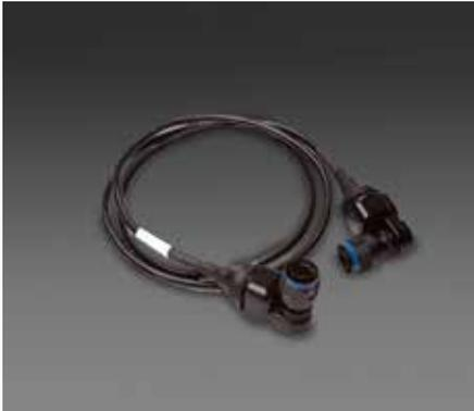
Moog Protokraft Cobra series active optoelectronic cable assemblies consist of optoelectronic transmitter and receiver functions integrated into an environmentally sealed unit with a D38999 / 26xB35PN electrical connector interface. The D38999 electrical interface to the Cobra series enables the use of high speed fiber optic cable links in applications exposed to extremely harsh environments.
