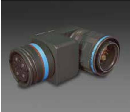
Moog Protokraft Proteus series media interface adapters consist of optoelectronic transmitter and receiver functions integrated into an external bulkhead mounted MIL-DTL-38999, Series III receptacle connector assembly. The optical transmitters are 850 nm VCSEL lasers.
