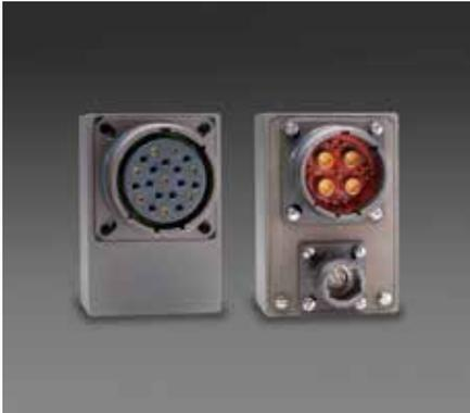
Moog Protokraft Falcon series dual DVI fiber optic transmitters or receivers consist of optoelectronic transmitter or receiver functions integrated into a bulkhead mounted MIL-DTL-38999 connector assembly. The optical transmitters are high output 850 nm VCSELs. The optical receivers consist of PIN and preamplifier assemblies and limiting postamplifiers for an easy link extension via fiber optics up to 500 m.
