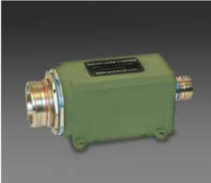
Moog Protokraft Viking series 4 and 1 Ethernet switches consist of 4x10/100/1000Base-T ports plus 1x1000Base-BX-U / D port in a wall or floor mounted inline MIL-DTL-38999 connector assembly.
