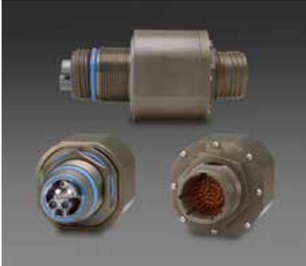
Moog Protokraft Mustang series dual fiber optic Ethernet media converters consist of optoelectronic transmitter and receiver functions integrated along with the 10/100Base-TX to 100Base-FX or 1000Base-T Ethernet electrical to 1000Base-LX or 1000Base-SX Ethernet optical media conversion circuitry into an environmentally sealed unit with a Jam Nut TFOCA II® optical connector interface.
