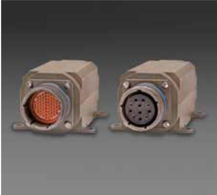
Moog Protokraft Viking series 4+2 port Copper + Fiber Ethernet switches consist of 4x 10/100/1000Base-T ports with autonegotiation and auto MDI/MDIX circuitry plus 2x 100Base-FX or 1000Base-SX ports in a wall or floor mounted inline MIL-DTL-38999 connector assembly.
