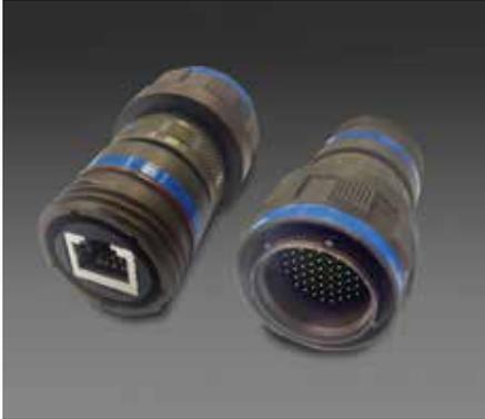
Moog Protokraft Gemini series media interface adapters consist of optoelectronic transmitter and receiver functions integrated into a bulkhead mounted MIL-DTL-38999, series III receptacle connector assembly. The optical transmitters are 850 nm VCSEL or 1310 nm FP lasers.
