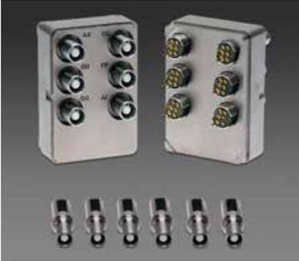
Moog Protokraft Magnum optoelectronic components integrate high performance fiber optic transmitter or receiver functions into a size 8 Quadrax cavity insert suitable for use in ARINC 600 / 404, EN 4165 or MIL-DTL-83527 connector bodies. Magnum optoelectronic transmitters/receivers consist of optoelectronic transmitter / receiver functions integrated into a printed circuit board mounted pin contact.
