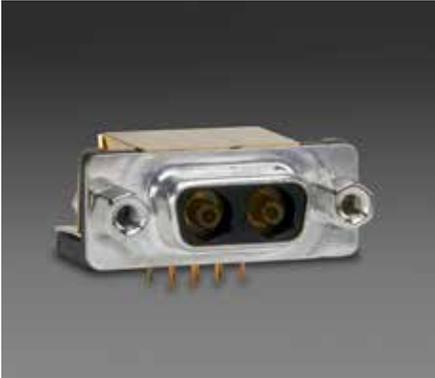
Moog Protokraft Direct 9 series D-Subminiature optical fiber transceivers consist of optoelectronic transmitter and receiver functions integrated into a printed circuit board mounted D-Sub / ARINC 801 compliant receptacle connector. The electrical interface to the Direct 9 series D-Sub optical transceiver is a solder pin field with the same PCB footprint as existing electrical 9 position D-Sub connectors.
