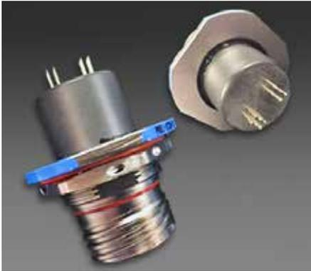
Moog Protokraft Cutlass series D38999 transceivers consist of optoelectronic transmitters and receivers functions integrated into a wall mount D38999 cylindrical connector. The optical transmitters are 850 nm VCSEL lasers. The transmitter input lines are driven with differential CML signals applied to the transmitter (TX+ and TX-) lines. Dual loop, temperature compensated, VCSEL drivers convert the transmitter input signals to suitable VCSEL bias and modulation currents.
