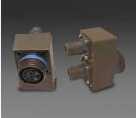
Moog Protokraft Mercury series Ethernet fiber optic media converters consist of optoelectronic single or dual transmitter and receiver functions integrated along with the 10/100Base-TX to 100Base-FX or 1000Base-T electrical to 1000Base-SX optical media conversion circuitry into an externally mounted MIL-DTL-38999 connector assembly.
