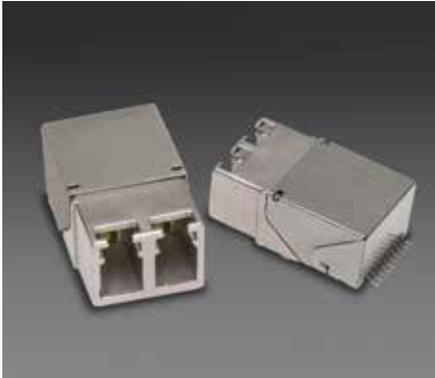
Moog Protokraft Razor series fiber optic transceivers with duplex LC interface consist of optoelectronic transmitter and receiver functions integrated into an surface mounted PCB assembly. The Razor series of fiber optic transceivers with duplex LC interfaces support Fast or Gigabit Ethernet, fiber channel, sFPDP, ARINC 818, ARINC 664 and many other protocols for multimode fiber optic links. All versions are fully compliant with the applicable IEEE or ANSI requirements.
