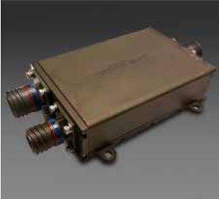
Moog Protokraft Eagle series 2xRS-170 to Ethernet converters grab images from 2xRS-170 sources and converts them to the Ethernet protocol and could compress them using H.264 for efficient video transport and distribution over Ethernet networks. These operations are performed with very low latency and jitter at the full GbE line rate.
