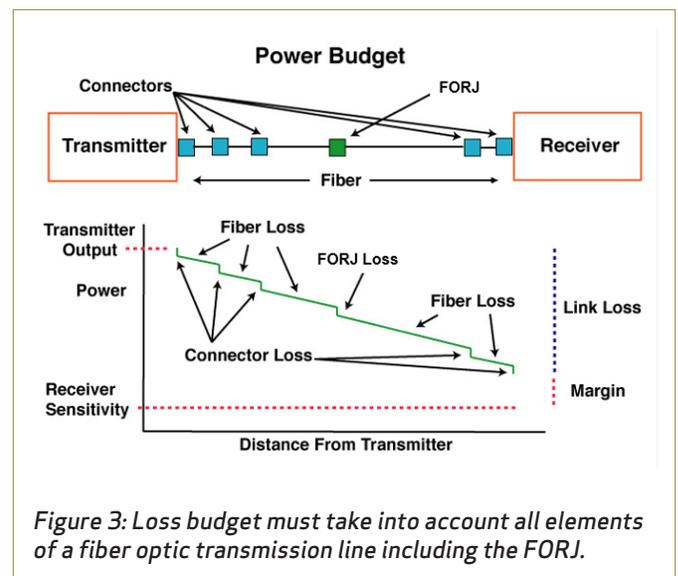
**Figure 3:** Loss budget must take into account all elements of a fiber optic transmission line including the FORJ.
