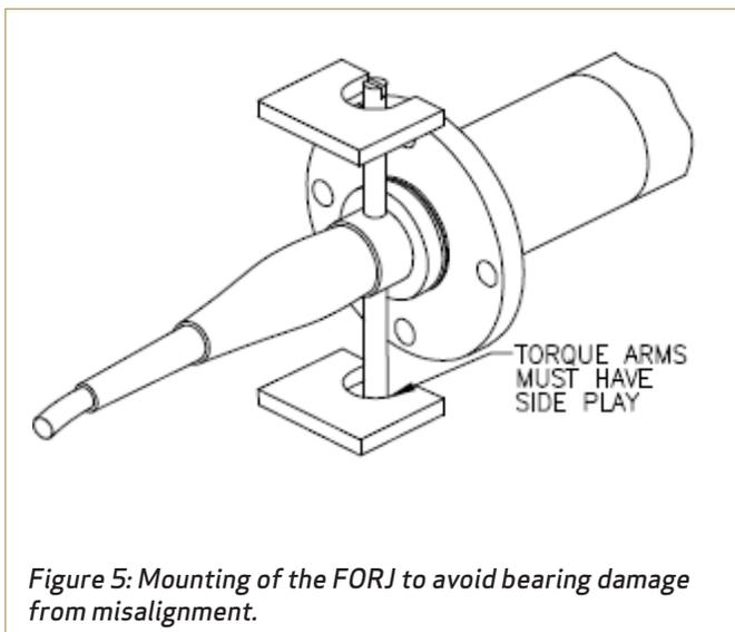
**Figure 5: Mounting of the FORJ to avoid bearing damage from misalignment.**
