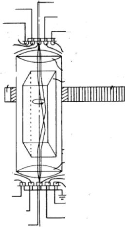
**Figure 7: Prism-based multi-pass FORJ concept. The prism rotating at 1/2 of the angular rotation speed in the opposite direction of the optical signals allows the signals to be aligned with the stationary fiber ends.**
