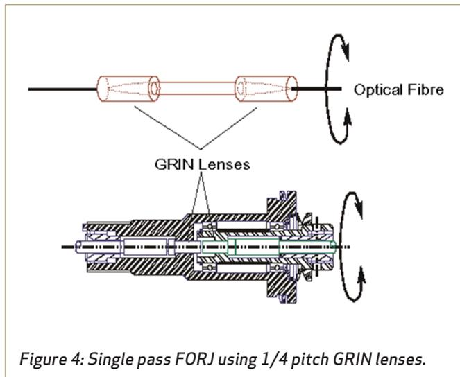
Figure 4: Single pass FORJ using 1/4 pitch GRIN lenses.
