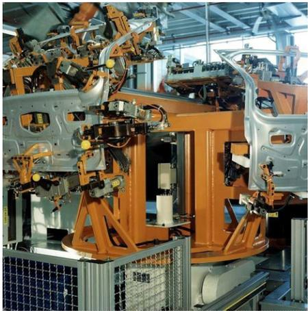
**Figure 2:** Complex automotive assembly turntable/robot has a fiber optic rotary joint in the center to transfer communication data. EMI isolation of fiber channel is critical in this application. Rotary joint provides power and signal slip rings as well as hydraulic power.
