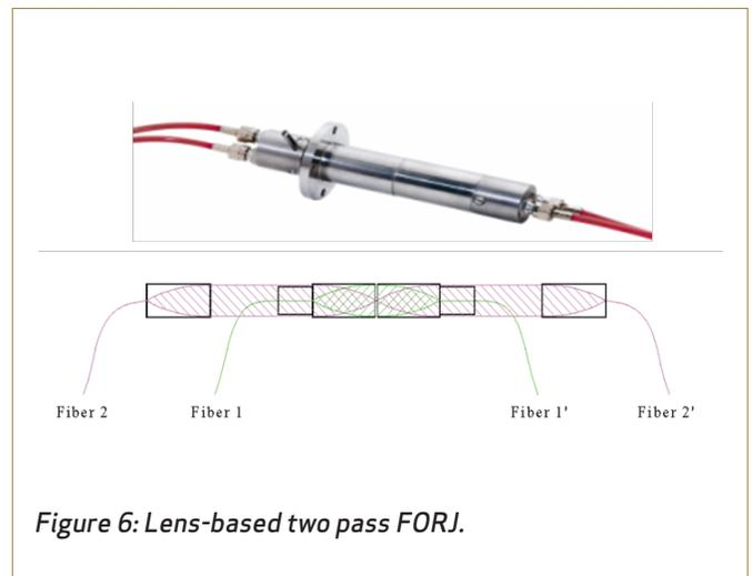
**Figure 6: Lens-based two pass FORJ.**
