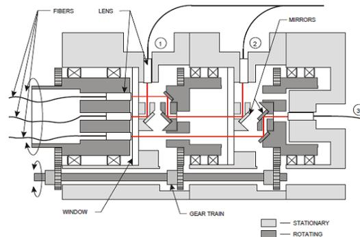
**Figure 8: A 2 cell (pass) mirror based approach is shown for a multipass FORJ. Cells can be added to achieve any number of desired passes up to about 10.**
