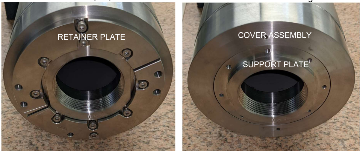
Figure 9 – RETAINER PLATE in place (left) and removed (right)
